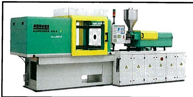
Figure 3. Allrounder A series MIM presses save energy
